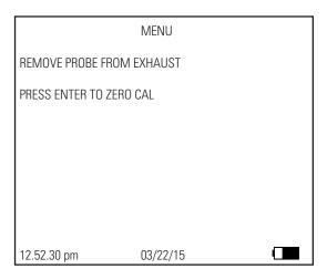
Ensure the probe is removed from the vehicle exhaust and is sampling fresh air, in the garage environment.
