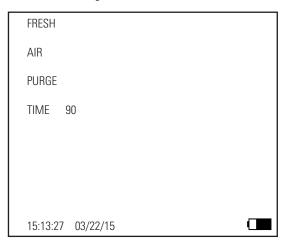
The time will count down in seconds to zero and is pre-set by the analyzer. During countdown the analyzer will initialize the measuring system, do not block the end of the probe or insert into or near the vehicle exhaust. It also displays some setup values including atmospheric pressure and internal ambient temperature.
